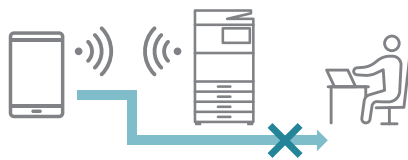
Mobile devices cannot access the company LAN via the MFD
